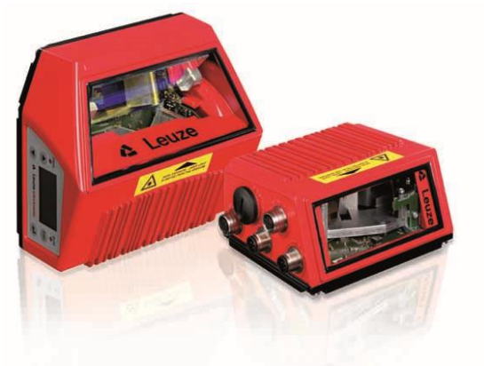
Figure 3. BCL 500i is a scanner family from Leuze electronic. The device on the left has an oscillating mirror attachment to increase the size of the reading field.
